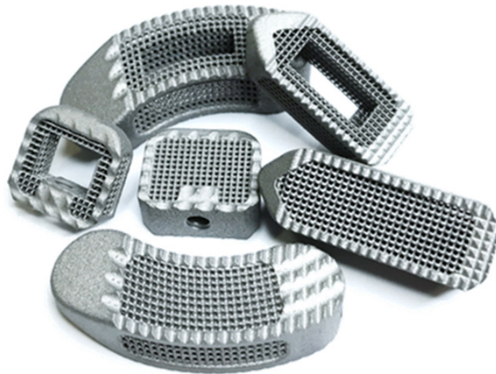
Fig. (1). Assortment of 3D-printed titanium spinal fusion cages featuring various designs and configurations tailored for different anatomical and surgical requirements. The collection includes cages designed for Posterior Lumbar Interbody Fusion (PLIF), Transforaminal Lumbar Interbody Fusion (TLIF), and Anterior Cervical Discectomy and Fusion (ACDF) procedures. The porous lattice structure is intended to enhance bone ingrowth, promote fusion, and provide improved stability, while the titanium material ensures biocompatibility and durability. The variety of shapes and sizes reflects the versatility of additive manufacturing in addressing the specific needs of spinal fusion surgery across different regions of the spine.
