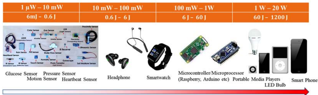
Fig. (1). Range of different sensors and electronic gadgets that can be powered using nanogenerators.
