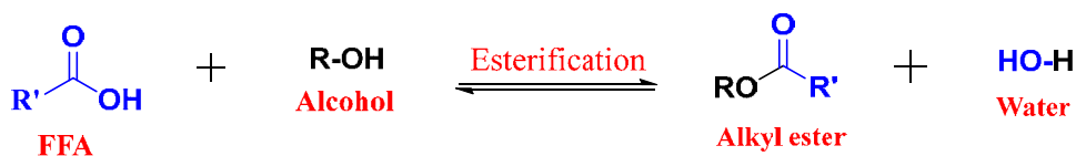
Fig. (2). Esterification of soybean oil to produce biodiesel (FAME).
