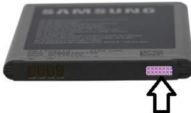
Fig. (2). Water-damaged battery [23].
