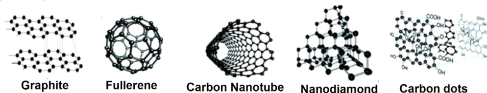
Fig. (1). Carbon nanoforms, Reproduced with permission from [3], under an open access Creative Common CC BY license.
