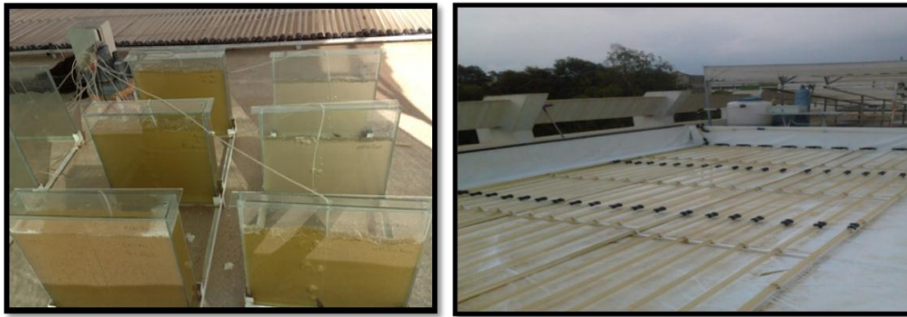
Fig. (2). Isochrysis aff. galbana cultures in tubular and flat-panel photobioreactors.
