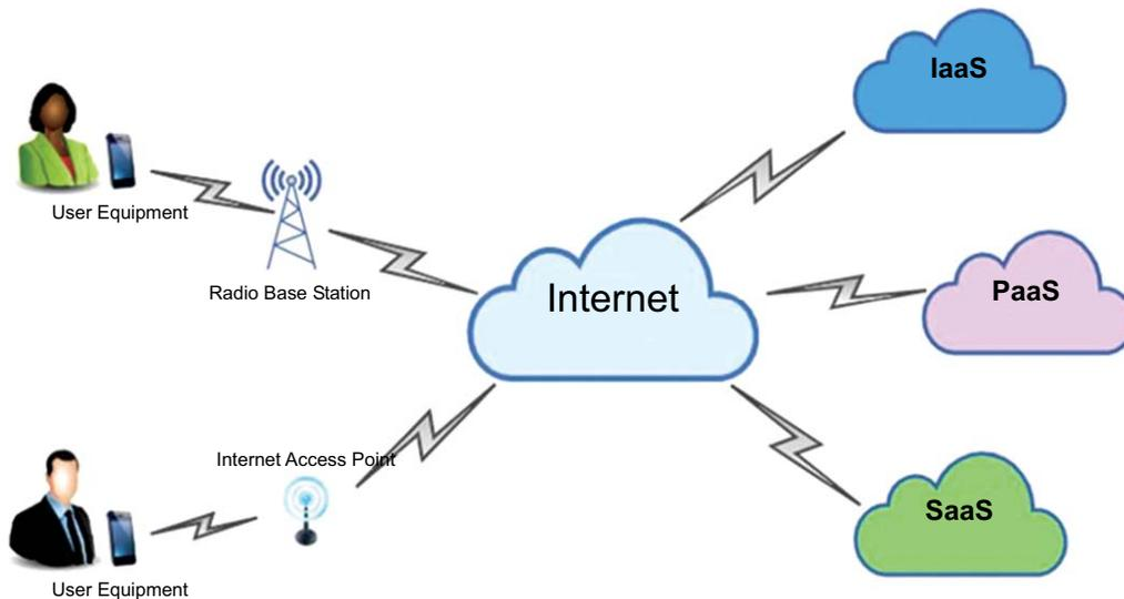
Fig. (1). Typical architecture of MCC services.
