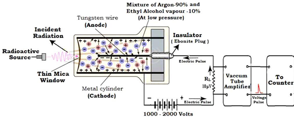
Fig. (4.1). Schematics of G. M. Counter.
