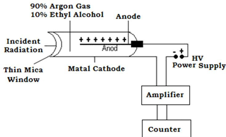
Fig. (4.2). Block diagram of G. M. Counter.
