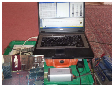
Fig. (1). High dynamic range ES-3000 Geometrics mobile station and Triaxial geophone used 4 HZ to drive soil and structure response of Abu Serga church.
