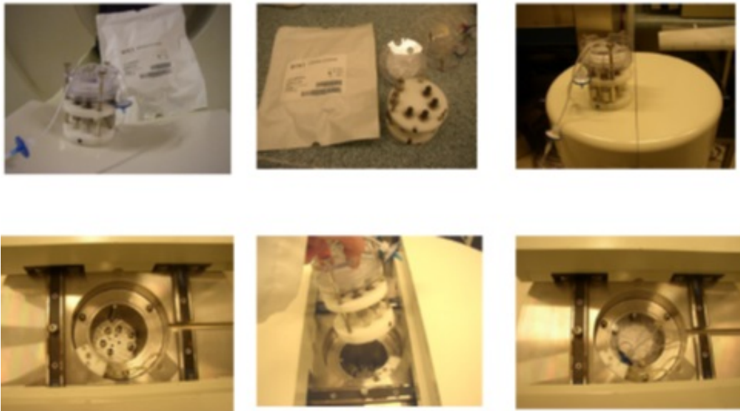
Fig. (2). GMP compatible ^{15}\text{O} -water delivery system components. The single use module with 2 semipermeable membranes is plugged in to the lead-shielded delivery system that is controlled remotely from the scanner control room by technicians. The device automatically delivers required bolus of ^{15}\text{O} -water to patient.
